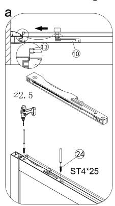
The first piston is located on the top of the fixed glass profile frame at the wall end as shown.
