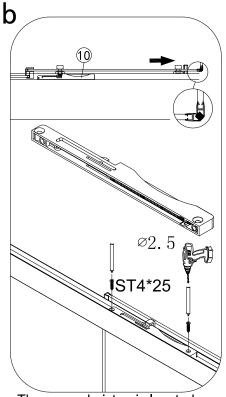
The second piston is located on the top of the fixed glass profile frame at the opposite end of the profile as shown.
